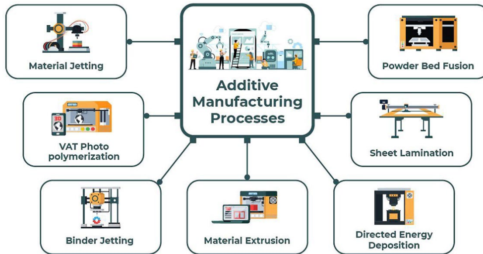
Figure 1: Additive can be broken down into seven core technologies. Within each, multiple materials including both plastics and metals can be processed. Source : https://manufacturing.report/articles/which-additive-manufacturing-process-is-right-for-you
